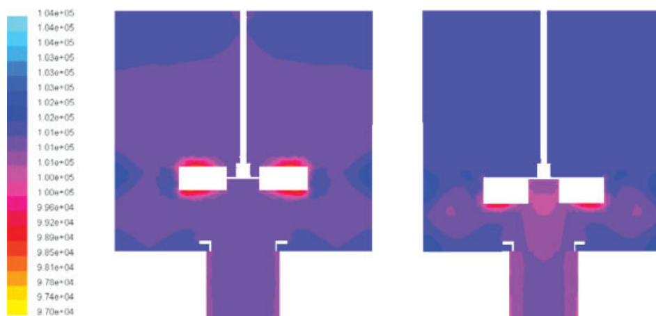
Figure 8. Relative pressure contours in a vertical central plane for RT (left) and TSTRRB (right) at Q = 0.002222 \text{ m}^3/\text{s} , N = 2.5 \text{ s}^{-1} .
